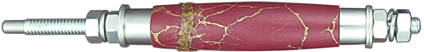
Blank After Filling Channel with Artisan Midnight Blaze Crushed Opal Inlay (Craft Supplies USA 1064380019)
