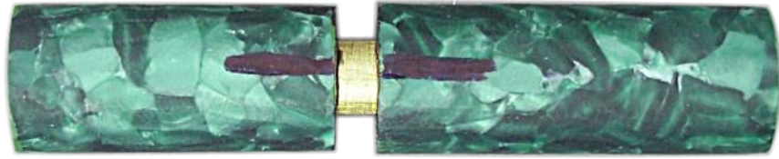
Acrylic Acetate Jade Green - Two Leftover Cutoffs Rough Turned to Align Pattern and Epoxied To 3/8" Brass Tube
