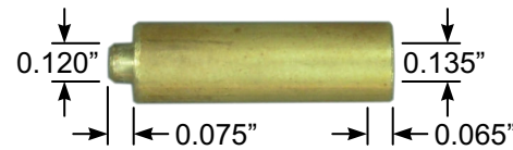
1/8" Magnet Installation Tool
