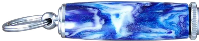
Artisan Deluxe Pill Holder in Chrome & DiamondCast Andromeda (Craft Supplies USA 1044430002 & Craft Supplies USA 1064360004) (Length Extended 0.5" Using 0.527" I.D. Brass Tube Turned Down to 0.577" O.D.) (McMaster-Carr 7782T641 Starting at 0.049" Wall Thickness)
