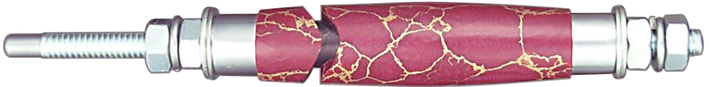
Single Wave Milled for Phoenix Rising Twist Pen in TruStone Maroon and Gold Matrix After Milling Channel for Crushed Opal Inlay with CNC Rotary Table (PSI PKRISEAB & PSI WXTS2134)
